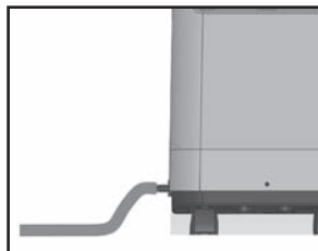
Figure 2a: Drain hose position
